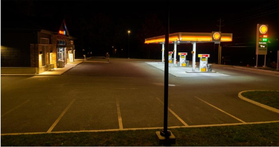
A new gas station and convenience store using 2200K LED luminaires from Lumenpulse. In Sherbrooke, commercial installations are required to use outdoor lights with a maximum of 10% of blue light (405-530nm) for parking and perimeter. The gas pump canopy can use lights emitting a maximum of 30% of blue light (equivalent to 4000K LED) for colour rendering.
